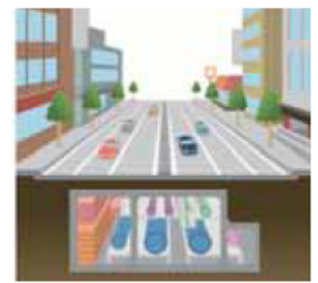
共同溝整備イメージ Picture showing the development of the utility tunnels
