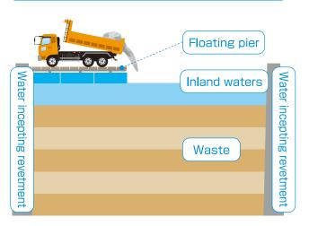
By relocating the floating pier, waste can be sent to landfill in a way that allows thin layers to be built up over a wide area.
