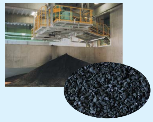
丸み付け処理後の路盤材空冷スラッグ Cold slag after rounding for road sub base coarse material
