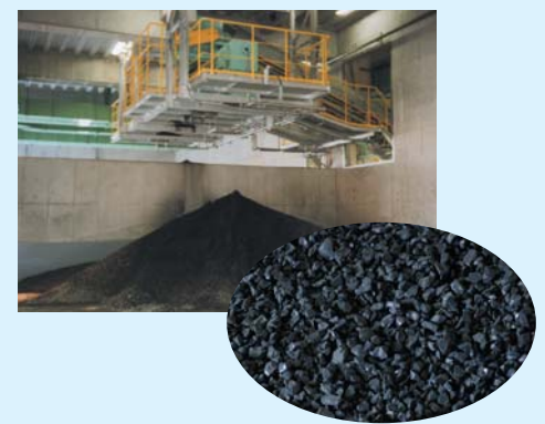
丸み付け処理後の路盤材空冷スラグ Cold slag after rounding for road sub base coarse material
