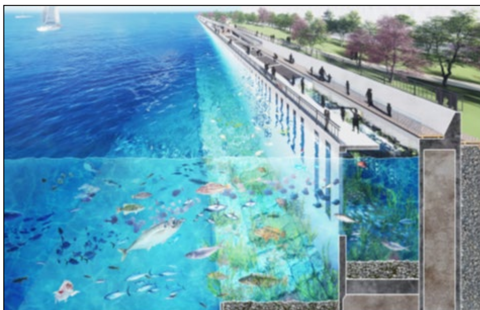
Figure 27: Image of a biosymbiotic seawall
