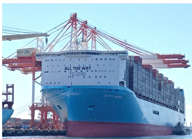
Methanol-fueled container ship “Alette Maersk”
