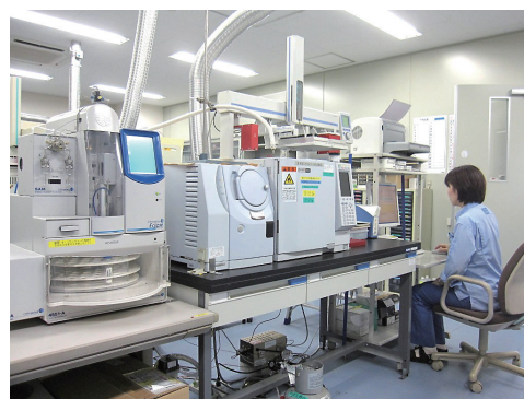
Organic substance examination using GC-MS
