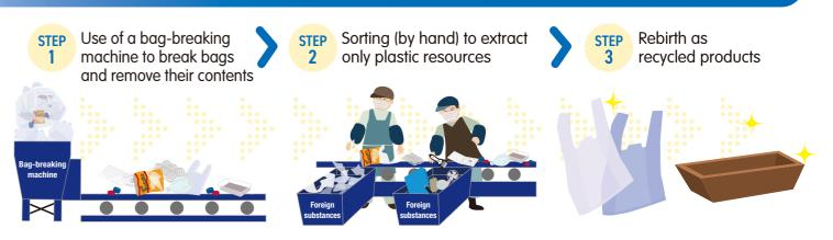
Intermediate processing facility (breaking of bags, removal of foreign substances, compression, and crating)
