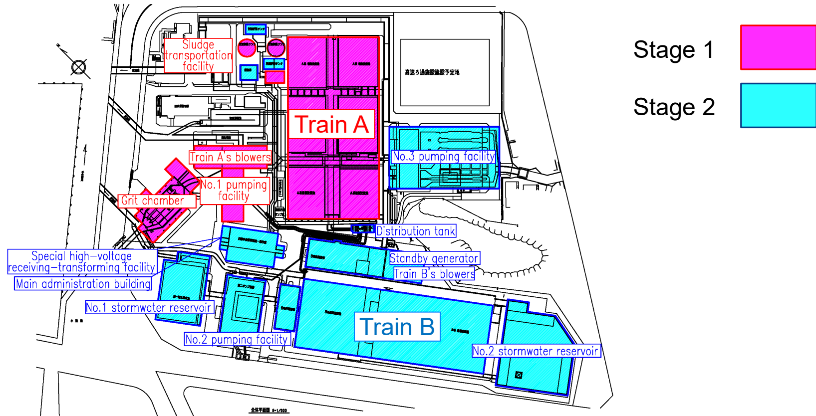
Figure 5 Classifying of Chubu WWTP
