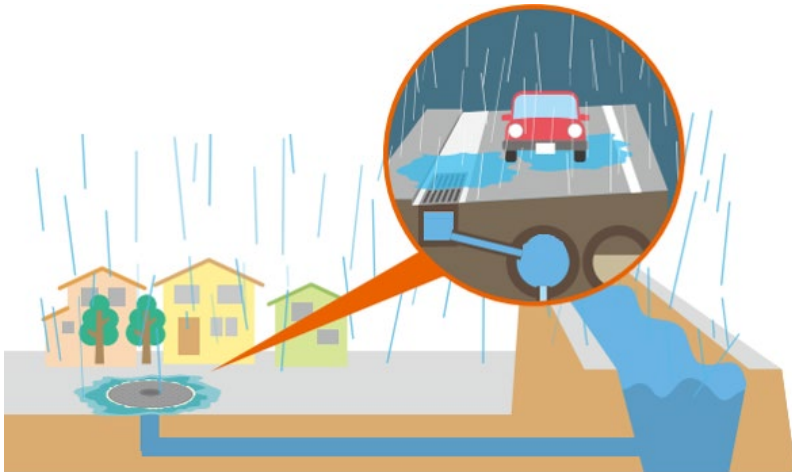
Lack of Sewer Capacity
