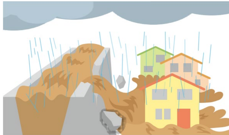
Breach of Flood Barrier
