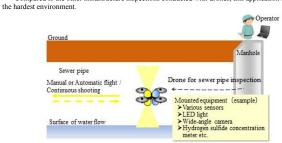
Figure 1 Diagram of inspection with a drone
