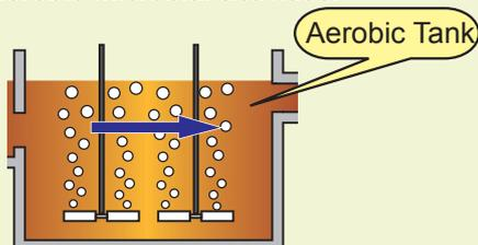
\*Aerobic Tank: Oxygenated with air supply
