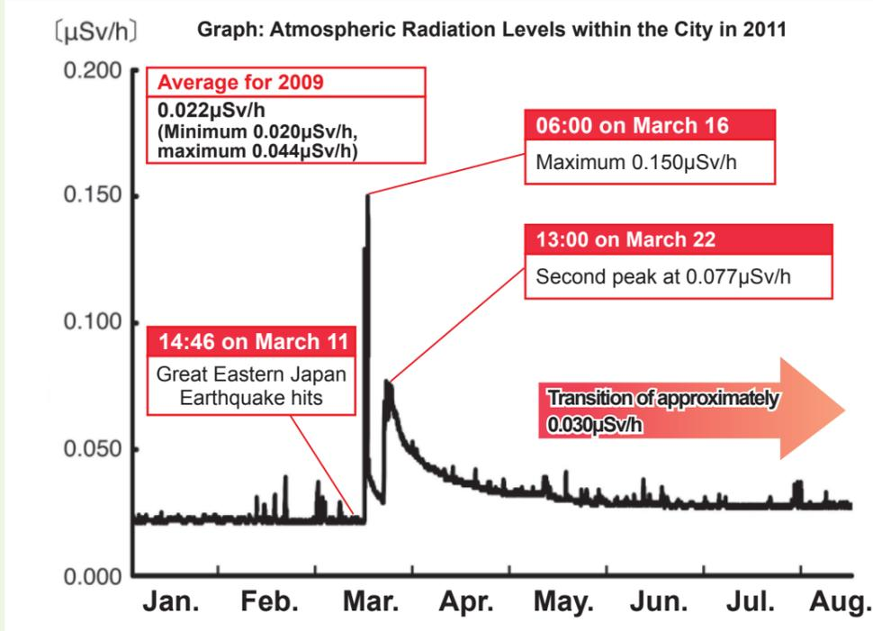
Measurements taken at the monitoring post (\*) located 23m above ground level at the Yokohama Institute of Environmental Sciences (Takigashira, Isogo-ku). Measurements in units of gray (Gy) are taken at the monitoring posts and converted into microsieverts at a rate of 1 nanogray/hour (nGy/h) = 0.001 microsievert/hour ( $\mu$ Sv/h).
