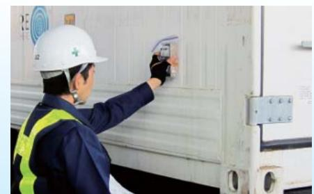
Scene of a cargo container being tested for radioactivity
