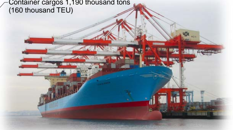
22-row mega gantry crane and containership growing in size
