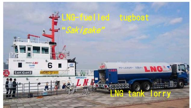
LNG-fuelled tugboat during LNG bunkering at the Port of Yokohama
